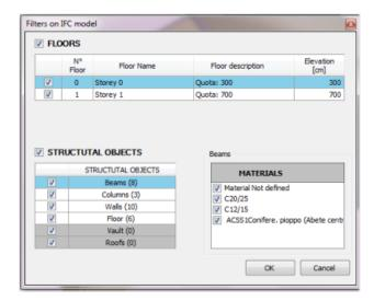
The first window shows all the active plans and all the active structural objects.
