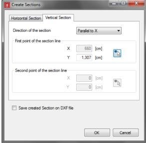
The position of the section can be entered manually by the user or by clicking on the desired point on the model.
