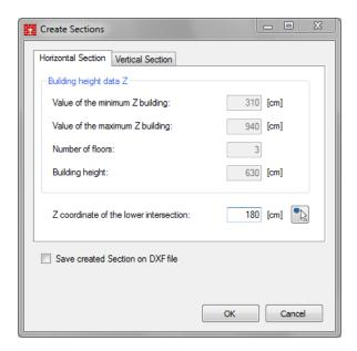
The created section is displayed in a new CAD area attached to the 3D model. If the auto saves on DXF file command is selected, the program displays a message saying that the file is created and displays the section. If the auto saves on DXF file command is not selected the section name assumes a default value (drawing1.vdml). In this case the section can be saved using the menu command File > Save As. You can create infinite sections.
